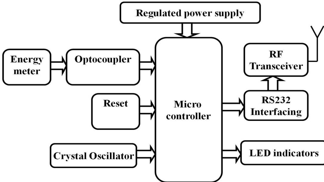
Wireless Energy Meter reading on hand-held device based on
